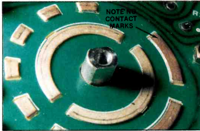
Figure 10. Inspection of the function switch in this as-is faulty meter revealed that some contact areas showed no sign of rubbing. Mechanical adjustment of the contacts was all that was needed to make it work.
