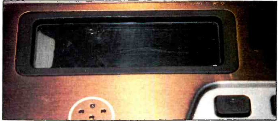
Figure 3. Don't buy an item with a cracked/blackened LCD display.
