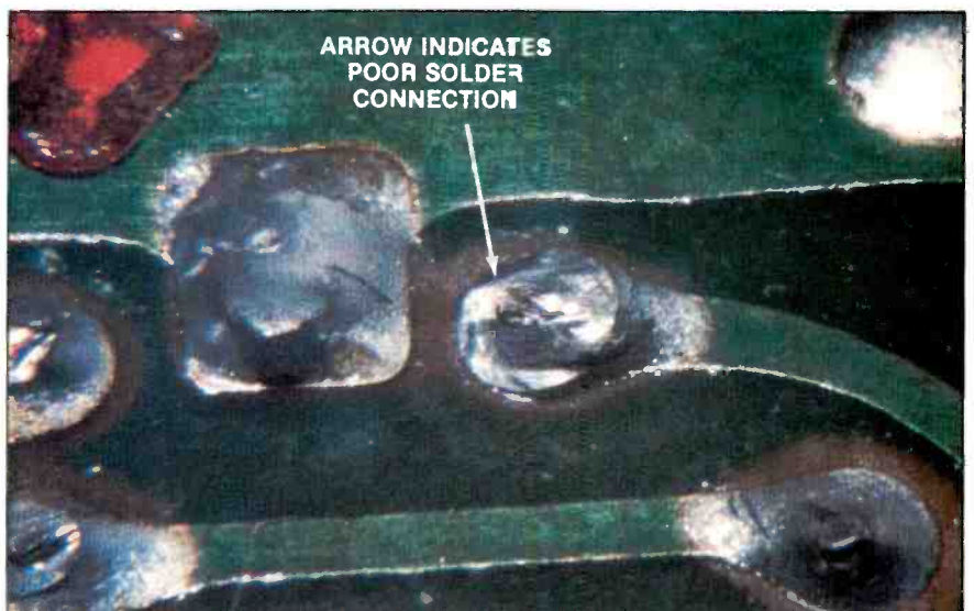
Figure 6. The portable AM radio in which this poor solder connection was found was completely dead until I tapped the printed-circuit board. Under magnification this connection was obviously bad. Reheating it brought the radio to life.
