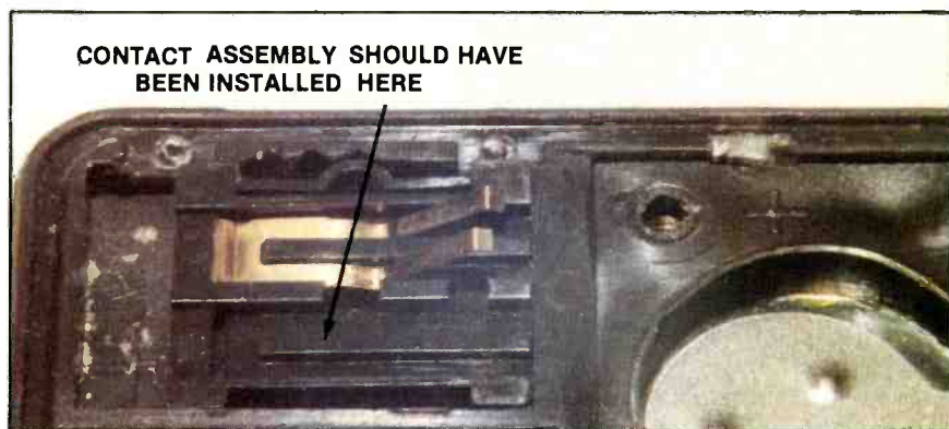
Figure 2. This calculator switch was assembled with the contact in the wrong slot.
