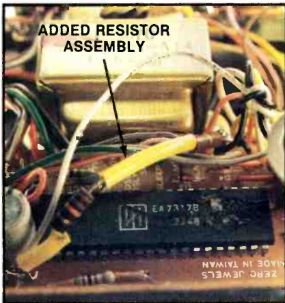
Figure 7. In this electronic clock, diagnosis showed that a pull-down resistor inside the IC was open. Adding a 14.2k \Omega resistor to the circuit outside the IC case restored proper operation.
