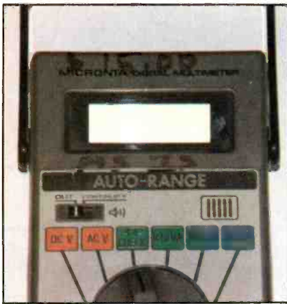
Figure 10. Inspection of the function switch in this as-is faulty meter revealed that some contact areas showed no sign of rubbing. Mechanical adjustment of the contacts was all that was needed to make it work.
