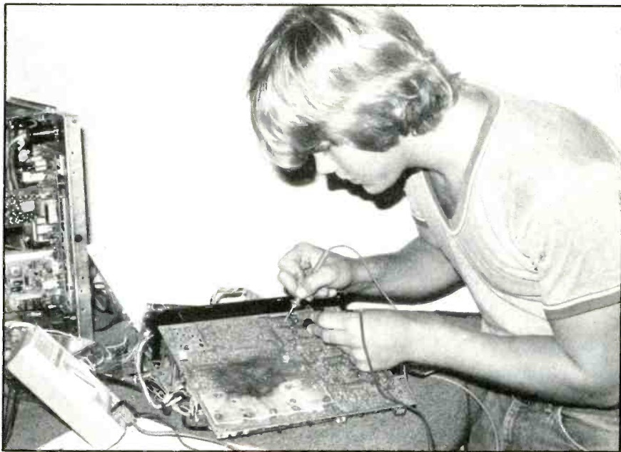
A TV technician is checking components that might have been damaged by lightning. Notice the large blackened area on this RCA circuit board. Individual defective components can be replaced, of course, but a circuit board that is badly carbonized over a large area calls for a new circuit board or discarding the entire receiver because of the huge costs involved.
