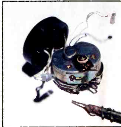
Figure 8. The control spring in this meter had broken, resulting in absence of movement. In such a case, a fine-tipped soldering iron, or one that has been modified as shown here, may be used to solder it back into place.
