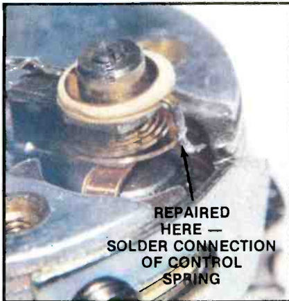
Figure 8. The control spring in this meter had broken, resulting in absence of movement. In such a case, a fine-tipped soldering iron, or one that has been modified as shown here, may be used to solder it back into place.
